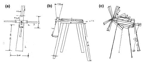
Fig. 3 Technical drawings of typical groups in the three settings—(a) TUM shows dimensions using conventions and numbering of parts to refer to steps in their procedural map; (b) TUE uses one-point lateral perspective with selective occlusion of a vane, a label (wire), dimensions with conventions; and (c) TRM shows multiple perspectives, X-ray depictions of vane and axle, selective abstraction of tower poles, and absence of end-lines in dimensions
