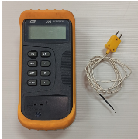
Figure 5.4: Chromel Alumel thermocouple with digital thermometer
