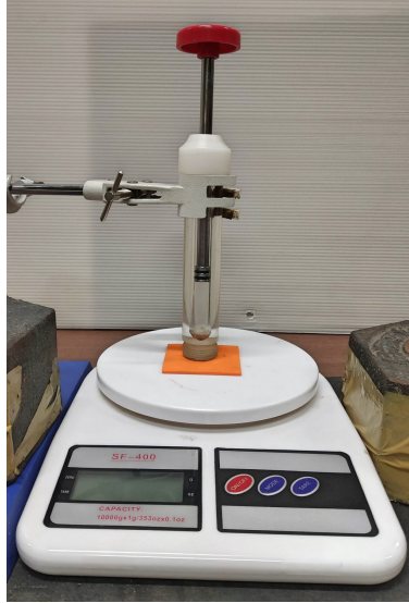
Figure 6.12: Arrangement for the pressure measurement during adiabatic compression
