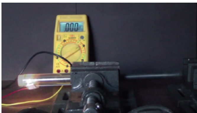
Figure 6.10: Adiabatic compression with heat flow reading displayed
