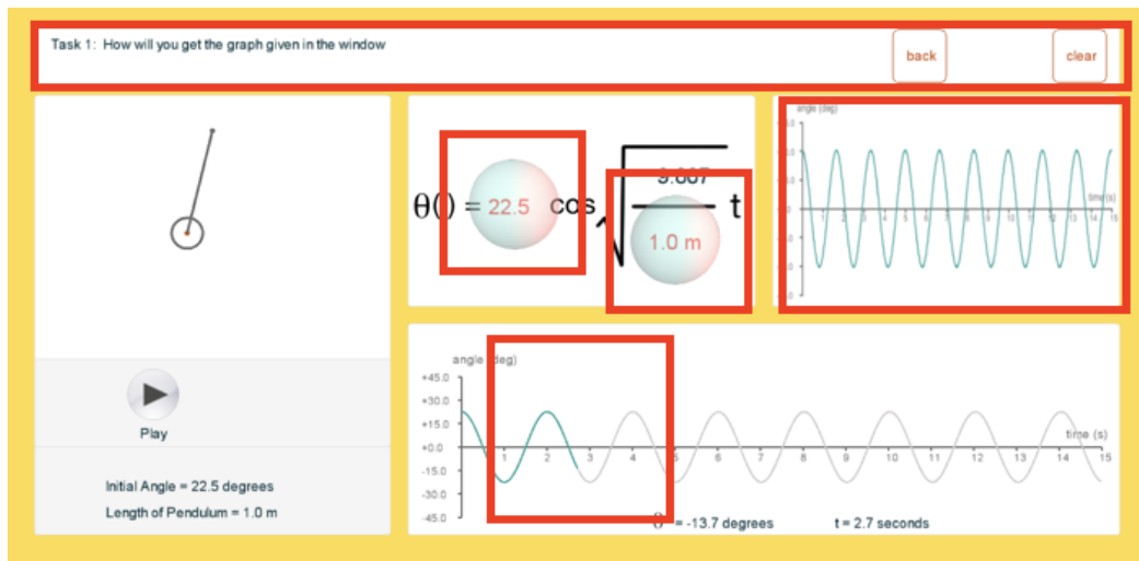
Figure 5.18 Screenshot of the computer interface version 2.1 with all 3 representational modes, a task and the “ghost” graph feature. Inside the red rectangular border on the top are instructions and back/next and clear buttons. In the centre of the screenshot inside the two different square-like red borders are the bevel buttons or bulged scrubbers (as opposed to sliders from the earlier interface version). Clicking and dragging the bevels would change respective values in the equation. Highlighted with a rectangular border below the back and clear buttons is a learning task. In the graph, blue-colored part of the curve is the curve being generated, while grey colored curve in the background is ‘ghost’ graph on which the blue colored curve is generated once the simulation is played. Only for screens 1-3, the ghost graph is manipulable by clicking and dragging either vertically (to change initial angle) or horizontally (to alter length). During the learning tasks, the graph cannot be manipulated.
