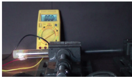
(b) Adiabatic compression with heat flow reading displayed
