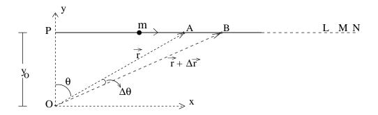
FIG. 5. A particle of mass m moving in a straight line path PABN with constant speed  $v_0$ . The origin O is not on the path. The particle travels from A to B in time  $\Delta t$  (Mashood and Singh, 2012b).
