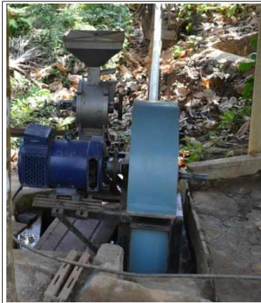
Fig. 7: GRI's domestic MHP system, also drives a flour mill
