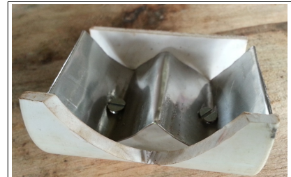
Fig. 55: Students' modified Pelton PVC bucket with a notch and W splitter
