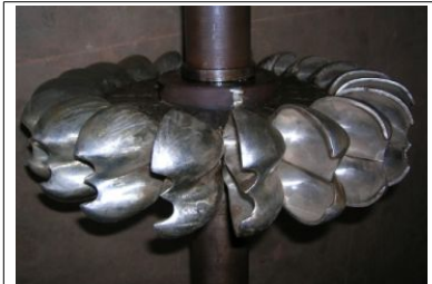
Fig. 54: Standard Pelton turbine with castings of split and notched buckets
