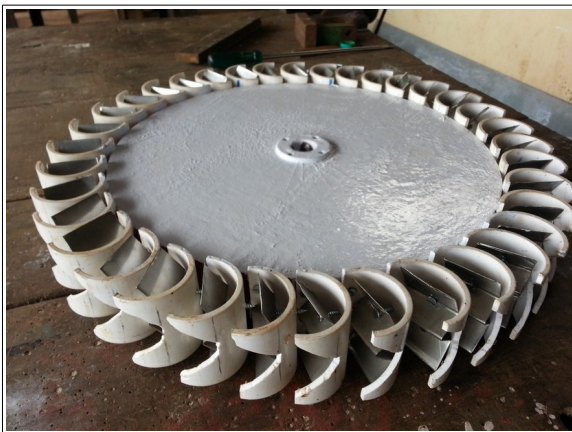
Fig. 30. ELs' innovative form of Pelton turbine wheel.
