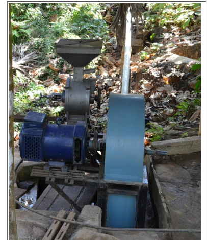
Fig. 6. GRI's domestic MHP system, also drives a flour mill.
