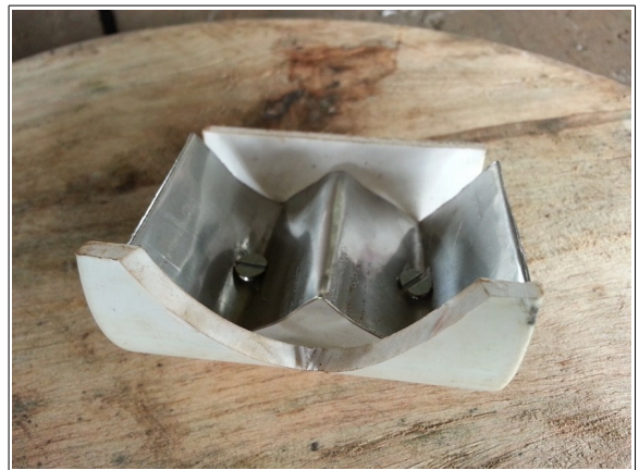
Fig. 31. ELs' innovative splitter for Pelton blade.
