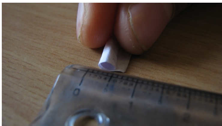
Figure 5.7: A student measuring mustard seed diameter by rolling a paper around it and later measuring the length of the roll.
