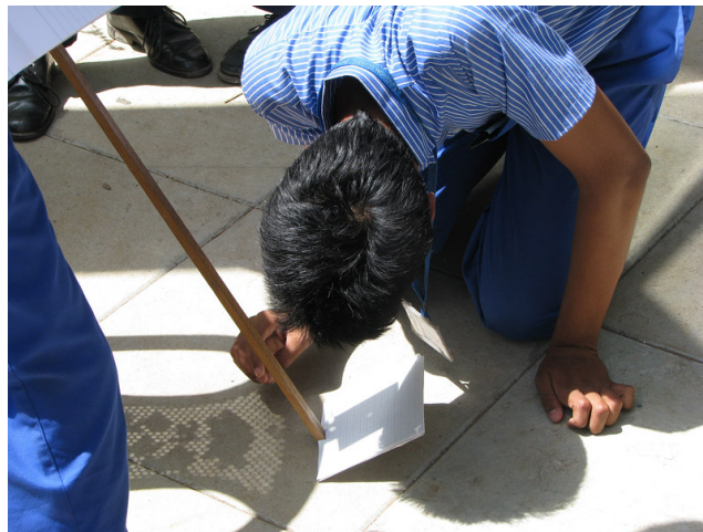
Figure 6.29: The Solar image obtained by the set-up as seen against the graph paper on the lower screen. We can see the Solar image in the centre of the square-shaped shadow of the upper pinhole box. The diameter of the image was read off the graph paper.
