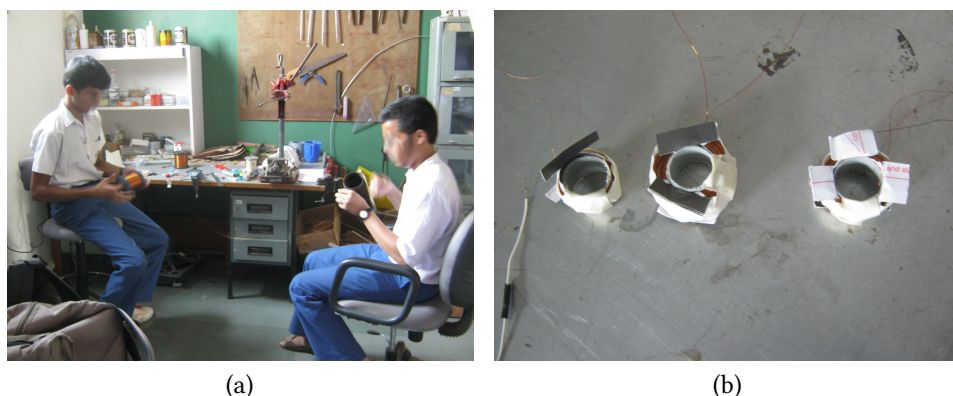
Figure 7.12: Students constructing coils with required parameters. (a) Winding wires on the coil, one student is holding the bundle of wire, while the other student is winding and counting the number of turns on the coil. (b) Some of the coils constructed by the students.
