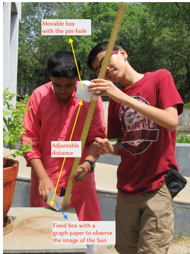
Figure 6.28: Students observing the solar image with the completed setup of the pinhole and the scale. The student on the right adjusts the movable box, while the other student observes the image of the Sun formed in the lower, fixed box.
