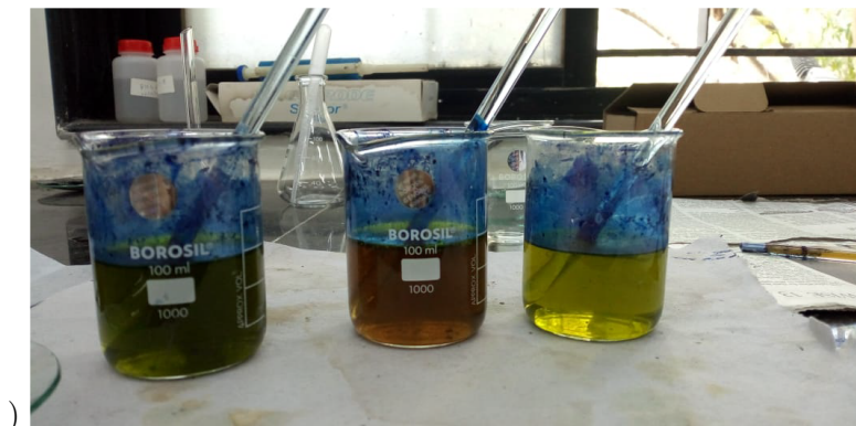
Figure 5.2: Leuco-indigo dye bath of different concentration(experiment on effect of varying percentage shade on yarn dyeing
