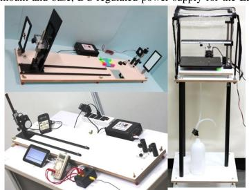
right reflectors (front coated mirrors), Screen (10 cm x 30 cm) with its mount, Plane mirror (10 cm x 10 cm), Sample I (helical spring), Sample II (double helix like pattern printed on glass plate), Plastic clips, Digital vernier calipers, Plastic scale (30 cm), Measuring tape (1.5 m), Light
